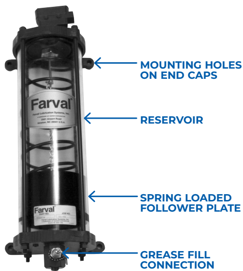
Grease Reservoir T30P5AC (Shown without pump attached)
